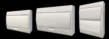
Purpose built for our circuit protection range, Wolverine switchboards deliver class leading protection and great features for your next resi install. Designed for indoor use, choose between 12, 18 & 24 module designs that are IK05 impact resistant and IP40 rated (from the front). Each board has a 100A rated assembly, neutral link and parts pack with 80A rated busbar, labels and pole fillers.
