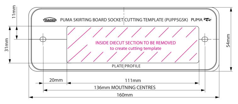
Note: Please ensure the above template is produced at exactly 100% scale of actual drawing to ensure correct fit.
