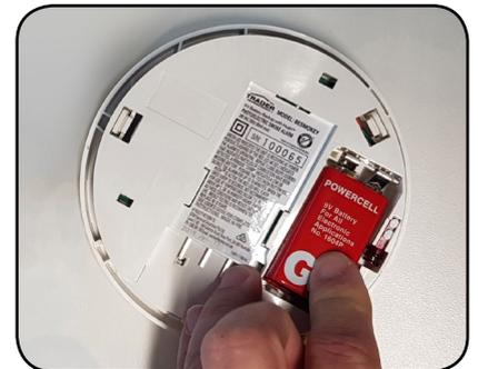
5. Fold in the red hinge arm and insert the battery ensuring the correct orientation.
