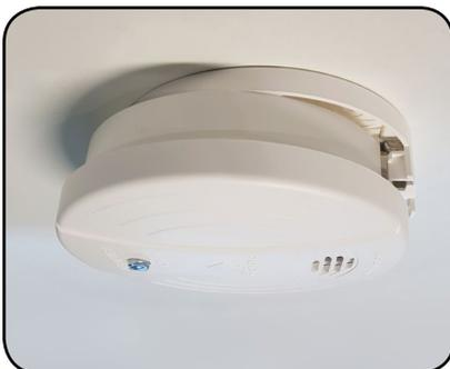
6. Slide the smoke detector together on the base plate until fully located in place.
