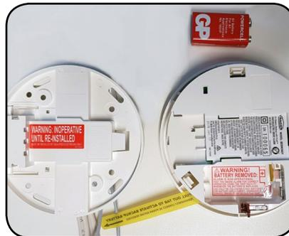
4. Once base is installed, remove the yellow tag covering the positive terminal in the battery chamber.
