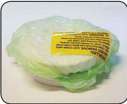
1. If installing in an area that is not under construction and contains excessive dust please remove the green shower cap and slide the base plate and main smoke detector model apart.
