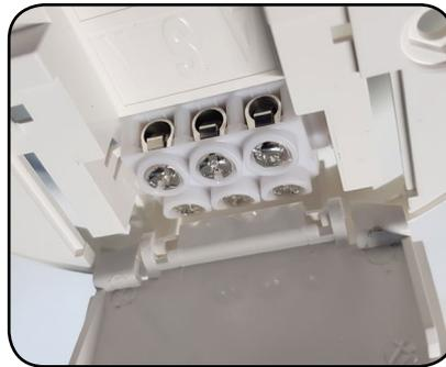
2. Open the terminal cover/and wire active/neutral into the terminals and if the smoke detector is being linked then utilize the switchwire terminal marked "S" for interconnection as per the instruction booklet. If Earth termination or looping is required a separate insulated connector such as Hyena HYICDS can be used.
