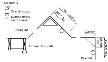
DEAD AIRSPACE AND PROPER MOUNTING OF SMOKE ALARMS ON SIDE WALLS
